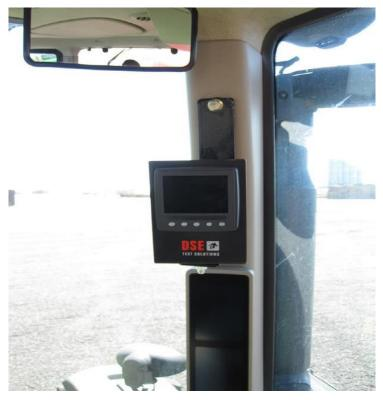
Avoid placing the Display in areas where it can be exposed to direct sunlight.
