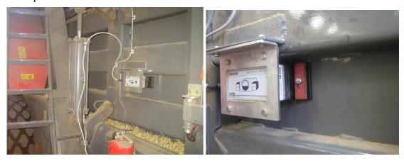
The picture below shows the inside of the channel. The metal strip welded to the wall before the TX/RX unit minimizes buildup of material around the TX/RX units that might damage them.
