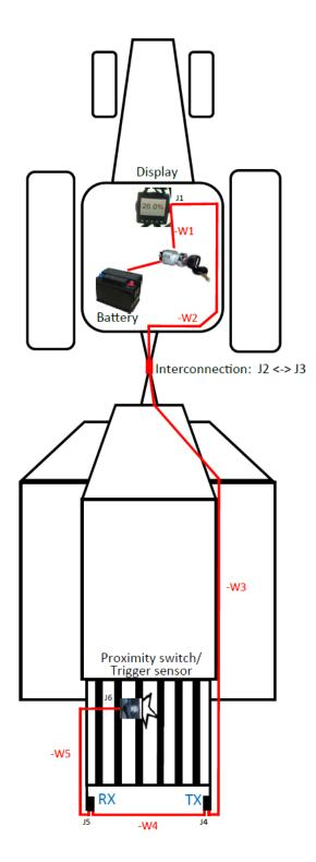
NB: Always connect DSE4200 to switched power (ACC), not directly to battery as shown in cable schematics
